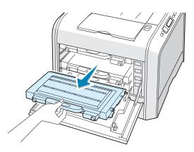
**CAUTION**: If you open the left cover for a few minutes, the imaging unit can be exposed to light. This causes damage to the imaging unit. Close the top and left cover should the setup need to be halted for any reason.
